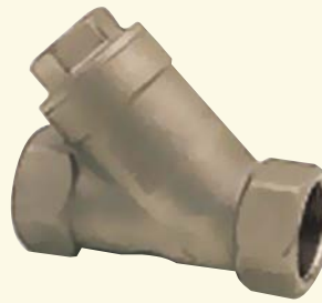
YSC-800 Y-Pattern Spring Check Valve • Size: 1/4" - 3" • 800 PSI • Body: CF8M
