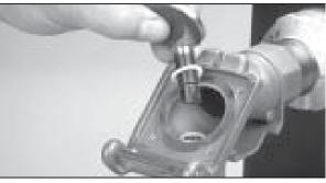
**3.** Put the o-ring over the disc stem. While holding the disc in the half turned position and taking caution not to scrape the disc edge against the coupler body, insert the disc stem into the stem seal and coupler body. Push the disc flush against the body.
