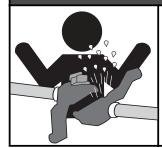
Piping systems must always be depressurized and drained before attempting disassembly and removal of any Dry Link Couplings.
