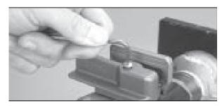
**1.** Using the proper size hex wrench, remove the pan head screw.
