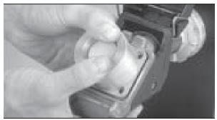
**4.** Install the seal ring assembly into the seal cavity around the disc by aligning the seal installation mandrel with the disc and pressing the seal ring into place with the seal installation sleeve (Installation sleeve available from Dry Link.)
