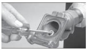
**3.** Remove the o-ring (or PTFE disc spacer, if equipped) and stem seal. Use caution not to scratch or score the coupler body in the disc seal area.
