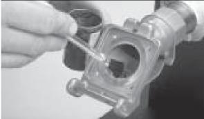
**2.** Apply an anti-seize compound into the stem hole in the adapterbody. Anti-seize should **not** be present in the stem seal area. Apply a light lubricant to the stem seal and the stem seal area of the adapter body.
