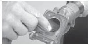
1. Clean the coupler body fully in the disc stem hole and the stem seal areas. Check for any corrosion or damage to the body in these areas.
