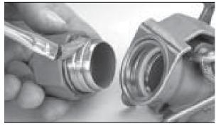
**5.** Using an anti-seize compound, lubricate the spline and spline groove on the swivel body.
