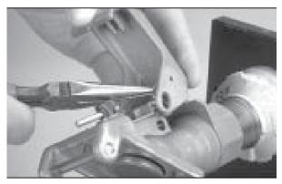
1. Insert the locking cap spring into the proper area in the body. Hold the locking cap in position and put the hooked open ends of the locking cap spring into the small holes provided in the locking cap. Push the spring's center leg behind the boss on the adapter.
