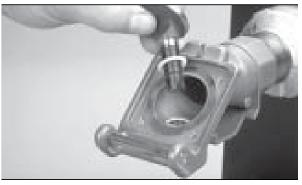
**3.** Put the o-ring over the disc stem. While holding the disc in the half turned position and taking caution not to scrape the disc edge against the adapter body, insert the disc stem into the stem seal and adapter body. Insert the disc until it is flush against the body.
