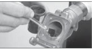
**2.** Apply an anti-seize compound into the stem hole in the coupler body. Anti-seize should **not** be present in the stem seal area. Use a silicone oil or grease to lubricate the stem seal and the stem seal area of the coupler body.
