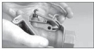
**5.** Twist and snake the bar out from the body opening. This may be difficult and will require a slight spreading of the open end of the locking bar.
