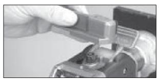
2. Remove the coupler lockout handle.
