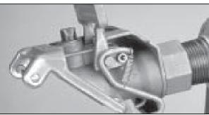
**4.** Complete assembly of the locking arm and locking bar by inserting the locking arm stand-off into the locking arm and through the corresponding hole in the coupler body. Check visually for proper assembly and function of the locking arm and locking bar.
