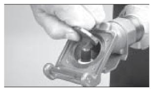
**3.** With the disc rotated a half turn, remove the retaining ring from the top of the disc stem and pull the disc out from the adapter body.
