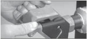
**2.** Remove the two socket head cap screws and the side panels. It is necessary to use an allen wrench on each screw. This will remove the first screw. It may be necessary to put the locking arm standoff in a soft jaw chuck to remove the second screw. Do not completely remove the locking arm standoff as this will disassemble the disc locking cap.
