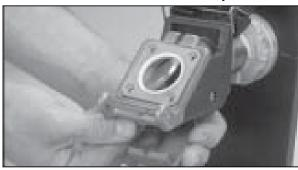
**2.** Adapter: Open the adapter disc by holding the hinged adapter stem locking cap down and turning the disc stem pin.
