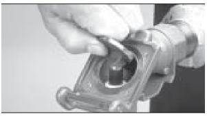
**2.** With the disc rotated a half turn or 180° from the closed position, remove the retaining ring from the top of the disc stem and pull the disc out from the coupler body.
