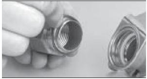
**4.** Place the external swivel o-ring seal over the swivel body.
