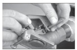
**2.** Pull the locking arm standoff out and remove the locking cap and locking cap spring.
