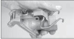
**4.** Remove the locking bar from the coupler body by first rotating the open end of the locking bar back over the swivel end of the coupler body.
