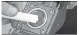
1. Remove the o-ring with a pointed tool. Pry and lift the "O" ring completely out of the groove. CAUTION: Permanent damage to the sealing surfaces may result if care is not taken during removal of the o-ring.
