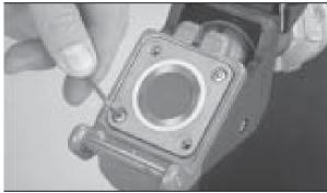
**1.** After depressurizing the system, remove the four socket head cap screws using the proper allen wrench.
