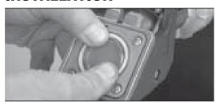
**2.** Press the new o-ring into the groove, beginning at one point and slowly working the o-ring into the seating area. A properly installed oring will extend less than ½2" above the disc face.
