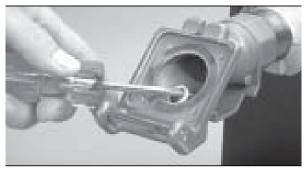
**4.** Remove the o-ring (or PTFE disc spacer, if equipped) and stem seal. Use caution not to scratch or score the adapter body in the disc seal area.
