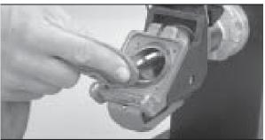
**1.** Clean the disc and body by wiping all sealing surfaces with a clean cloth. Be sure that no residue remains on the disc faces.
