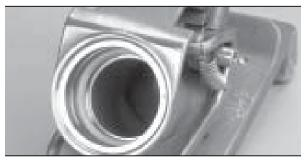
**3.** Place the internal swivel seal into the coupler body with the seal spring facing into the body. Take caution not to bend or fold the swivel seal.
