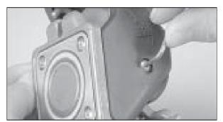
**2.** Remove the two socket head cap screws and the side panels. It is necessary to use an allen wrench on each screw. This will remove the first screw. It may be necessary to put the locking arm standoff in a soft jaw chuck to remove the second screw. Do not remove the locking arm stand-off completely as this will disassemble the disc locking cap.
