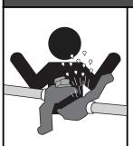
Piping systems must always be depressurized and drained before attempting disassembly and removal of any Dry Link piping products.
