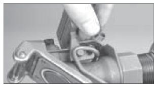
2. Insert the locking arm spring into position.
