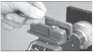
**1.** Reassemble the coupler lockout handle using the pan head screw. Do not over-tighten the screw. Test handle to ensure proper function of the unit.
