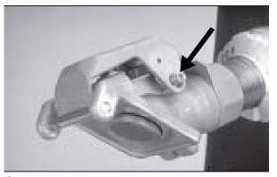
**2.** Insert the locking arm standoff into the locking cap. Install standoff through the locking cap spring loops to the hole in the adapter body and through the spring loops and back out the locking cap. Test locking arm to ensure proper assembly and function.
