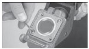
**5.** Re-install and tighten the screws with the proper allen wrench.
