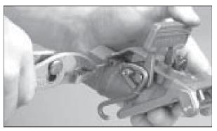
**1.** Remove the coupler cover and side panels (See Kit L for instructions). Using pliers, grab the end of the spline and pull the spline completely out of the coupler body and discard.
