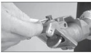
**5.** With the disc rotated a half turn or 180° from the closed position, insert the disc retaining pin into the stem hole. Use a hammer and lightly tap the pin into position.
