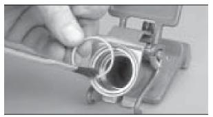
2. Using a silicone oil or grease, lightly lubricate the seals.
